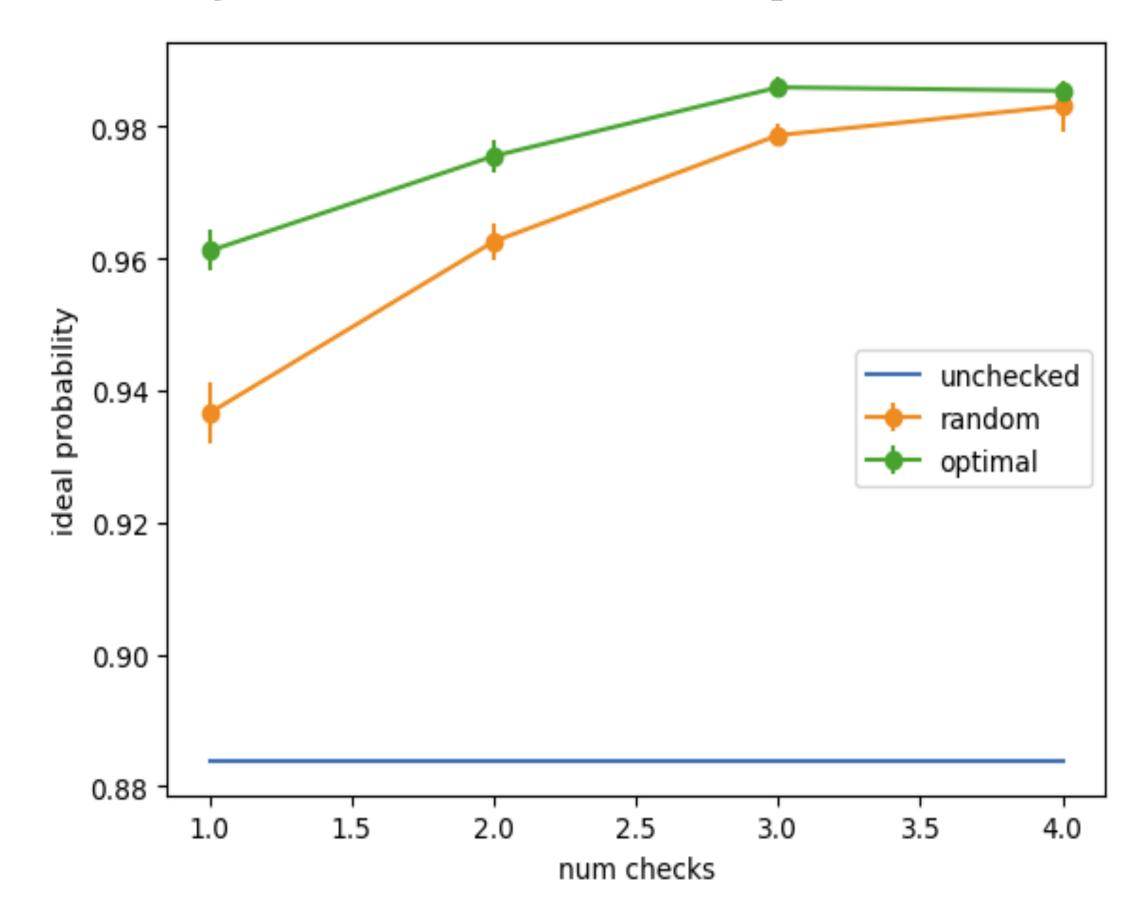
Adding more checks increases the set of errors which can be detected, increasing the ideal output probability towards the target value of 1.
