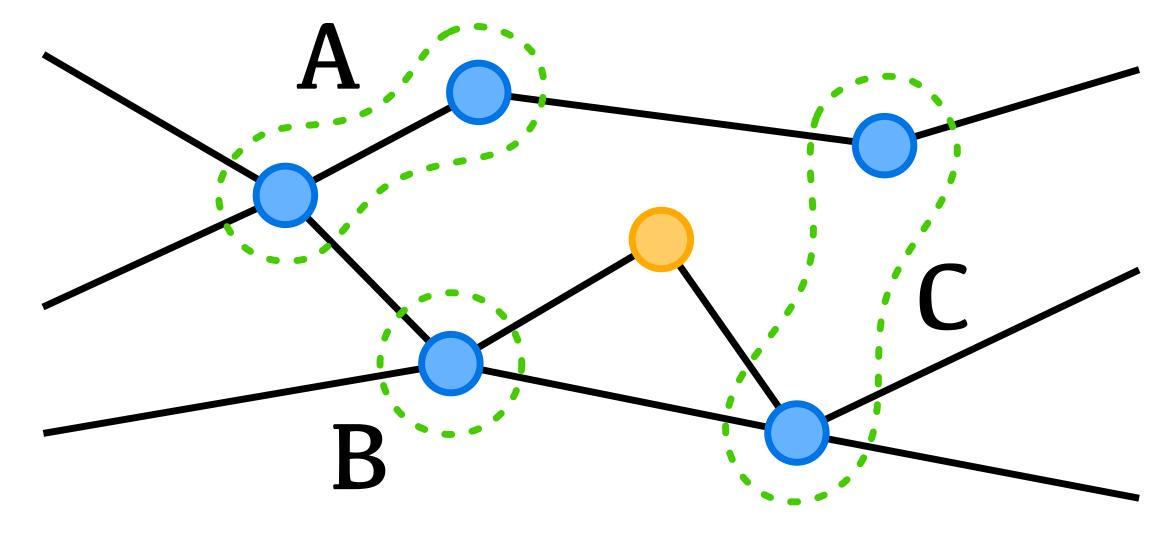
Subgraphs can be merged when the merged subgraph is convex. Convexity can be checked efficiently by checking paths between the subgraphs to be merged. A and B can be merged, but not B and C.
