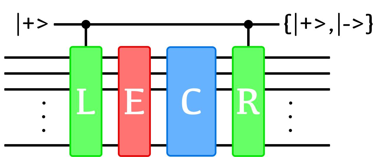
If E is uniformly distributed, and L is picked uniformly at random, 50% of errors are detected. This technique is called Coherent Pauli Checks (CPC); see "Single-shot error mitigation by coherent Pauli checks"
